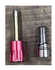
2) Use number 6 hex tool to screw in and tighten the inside screw to the bottom of the fork.
